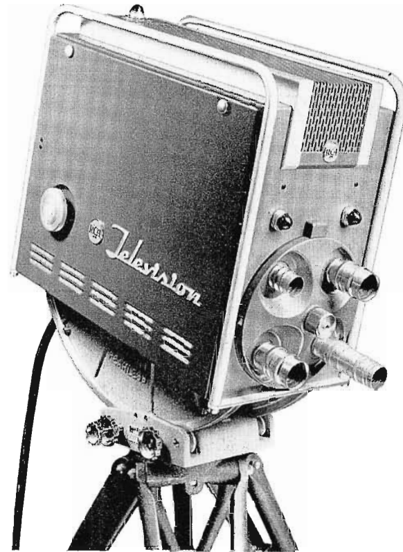
FIG. 5. Large 9-inch, 4-lens, broadcast-type turret is used on TK-15.
