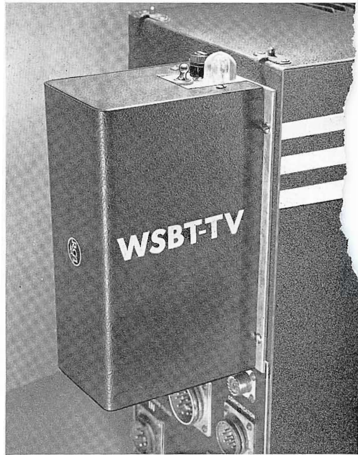
FIG. 1. Rear view of TK-31 camera control unit showing placement of the orbiter generator control box.
