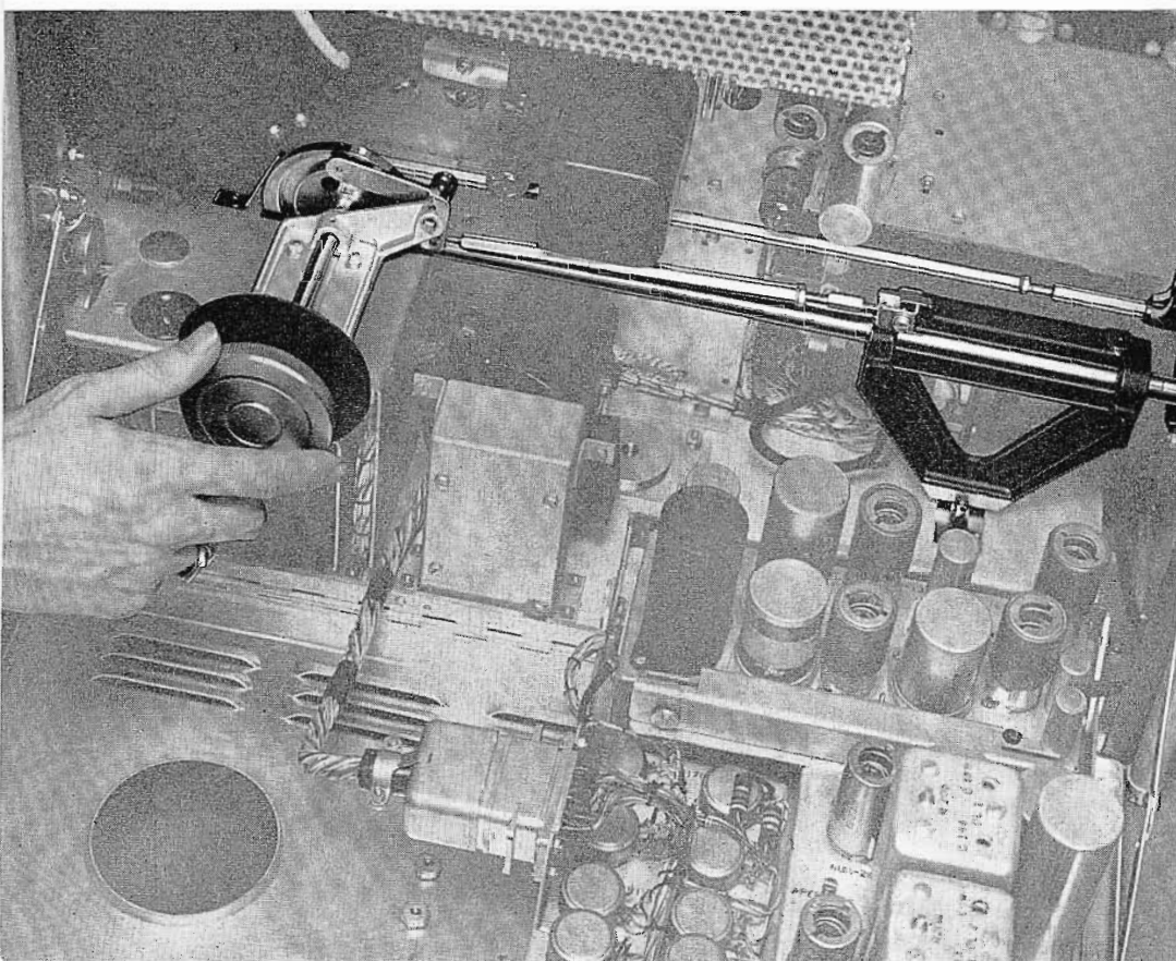
FIG. 10. Direct-drive focus control provides precision focusing. A 300-degree turn carries through complete focus range.
