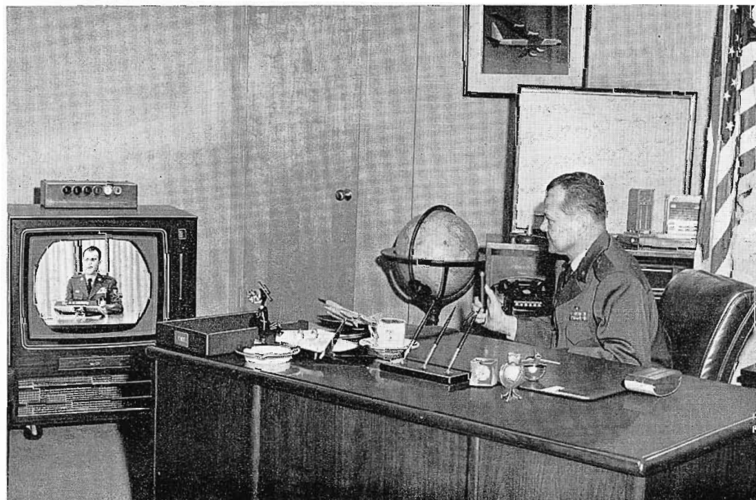
FIG. 16. A typical subscriber location at SAC. Here, Maj. Gen. Edmundson, SAC Director of Operations, watches a briefing in his office. Note microphone in his right hand, provided for conversing with control personnel.
