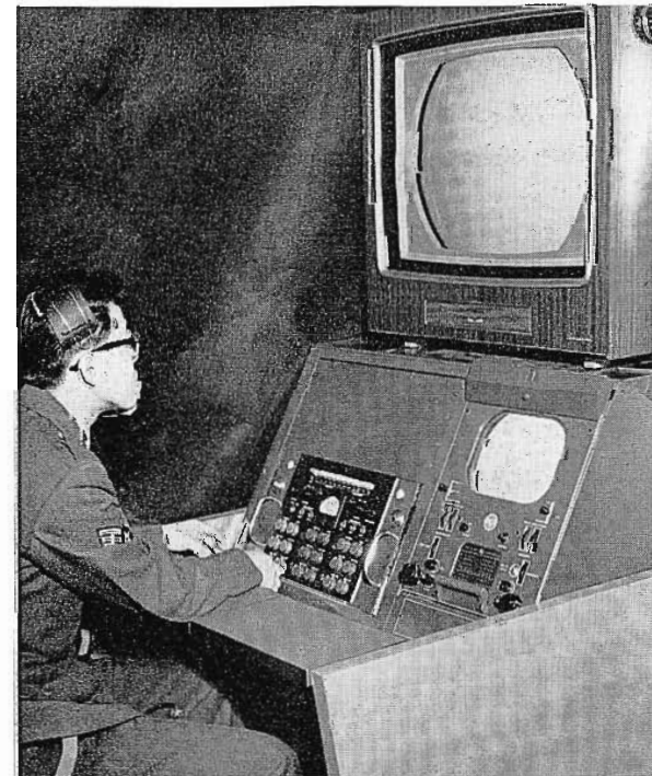
FIG. 11. Controls for Color TV Camera No. 1 are located in a separate corner of the control room. The operator can see the image in black and white on the master monitor as well as view the color presentation on the 21-inch modified color TV receiver positioned on top of the console.
