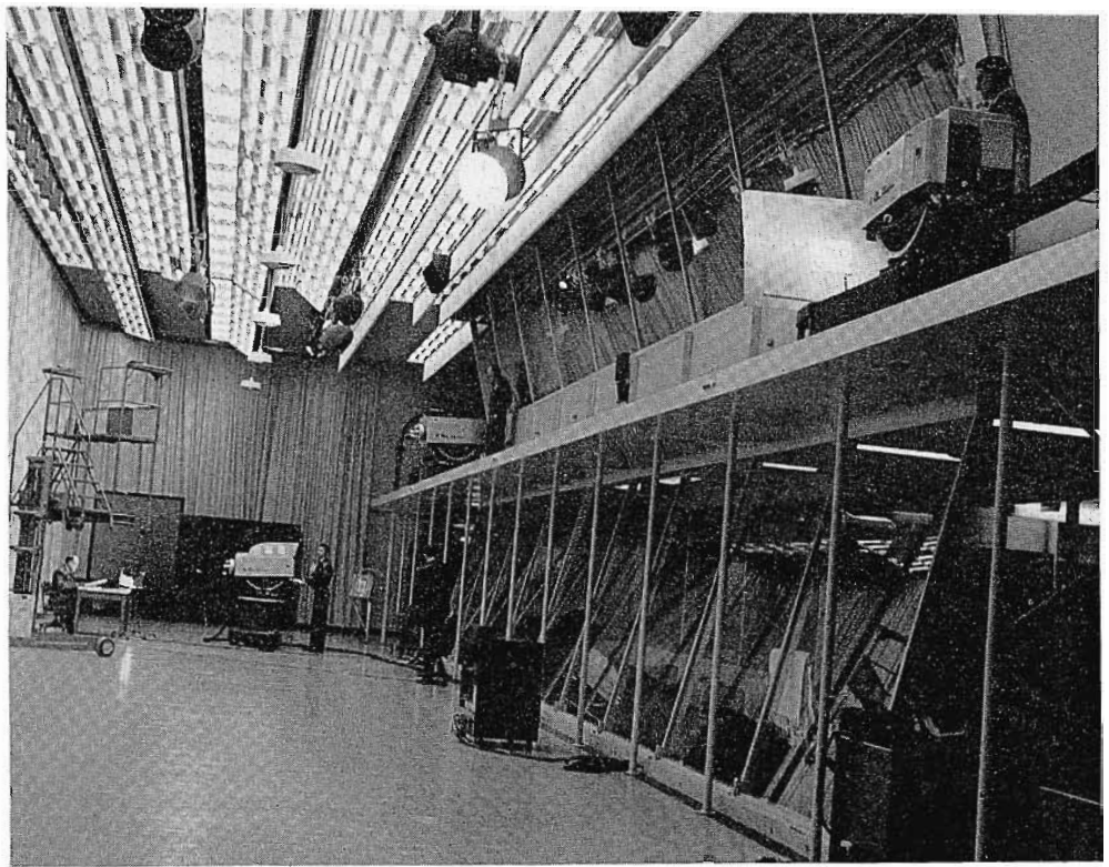
FIG. 14. A briefing emanates from the Operations Map Room. The floor camera (TK-41) is focused on the briefer. One track camera (right) is trained on a small chart supplementing the main briefing. Banks of fluorescents provide much of the lighting required for televised briefings.
