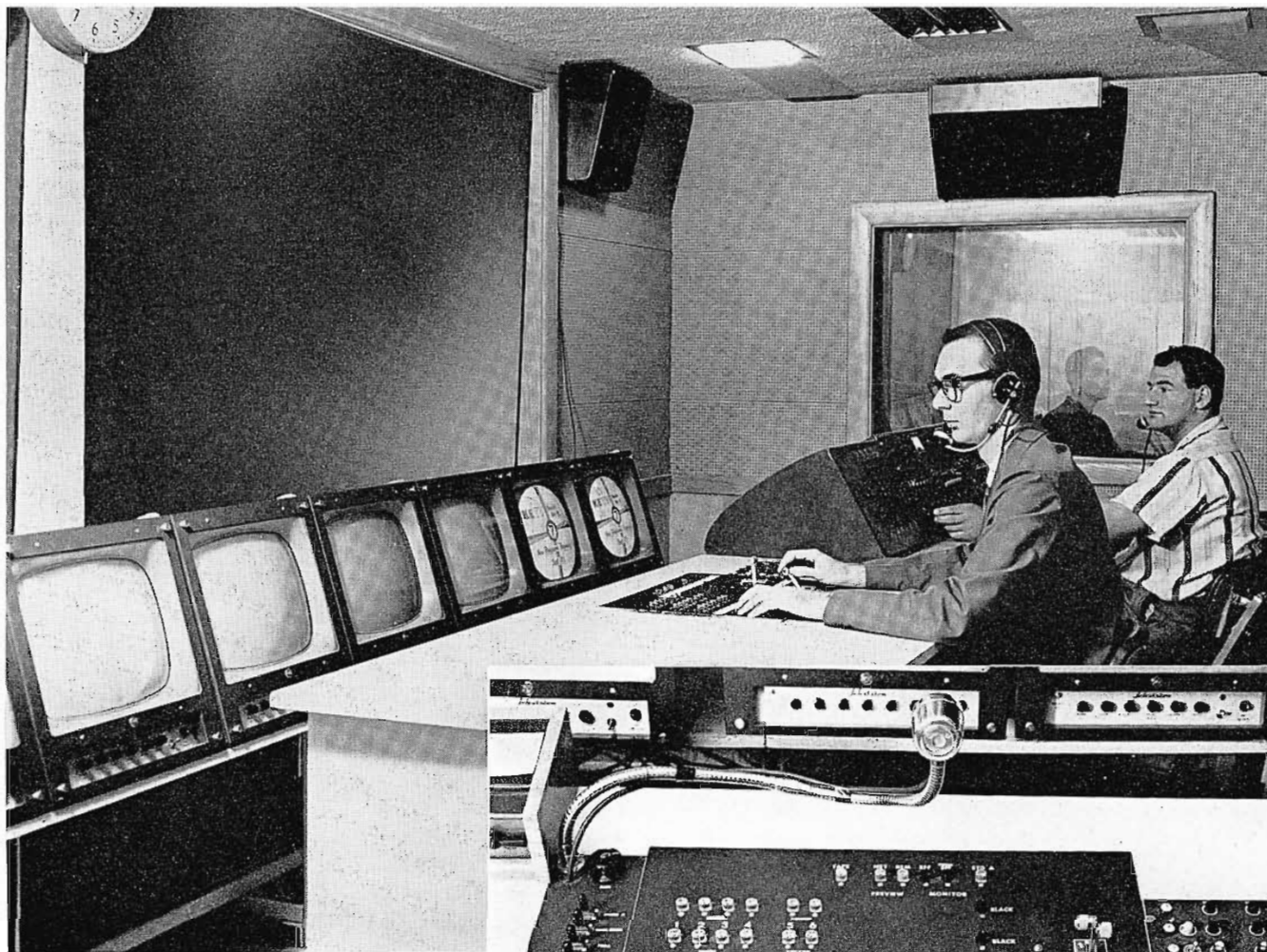
FIG. 10. Live studio control is nerve center of operations when KETV is producing a show from its studio. The producer-director has a bank of controls at hand, as well as the audio man. Window at rear looks into announcer booth.
